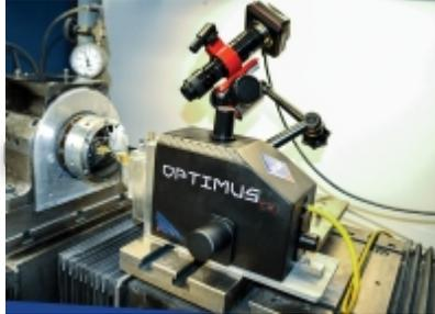
Micro-LAM's Optimus employs a high-power laser to soften brittle material like silicon before it is cut by a diamond-tipped cutting tool. The product can be retrofitted onto a company's existing CNC machine in roughly two hours and can increase productivity by as much as 500 percent, said company founder Deepak Ravindra. Going forward, Ravindra plans to develop Optimus to allow it to machine materials including sapphire and glass.
